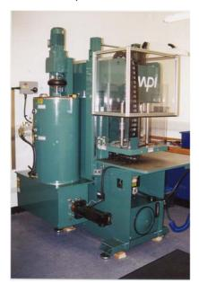
The injection press is a 22 tonne 'C' frame construction with side and bottom injection facilities. The wax tank has cooling as well as the
